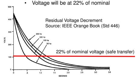
Figure 4-14—Induction motor open-circuit voltage decay (based on constant speed)
