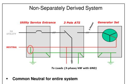
• Neutral is connected to ground at the Service, Not at the generator set
