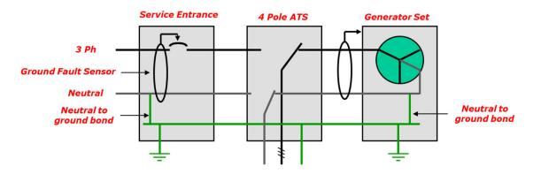
In order to meet both rules when connected to either the normal or the emergency source the neutral must be switched using a 4-pole transfer switch
