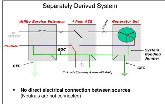
Generator Neutral is solidly bonded to Ground - Jumper
