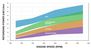
\*Demonstrated engine brake performance ranges from various engine tests and simulation results
