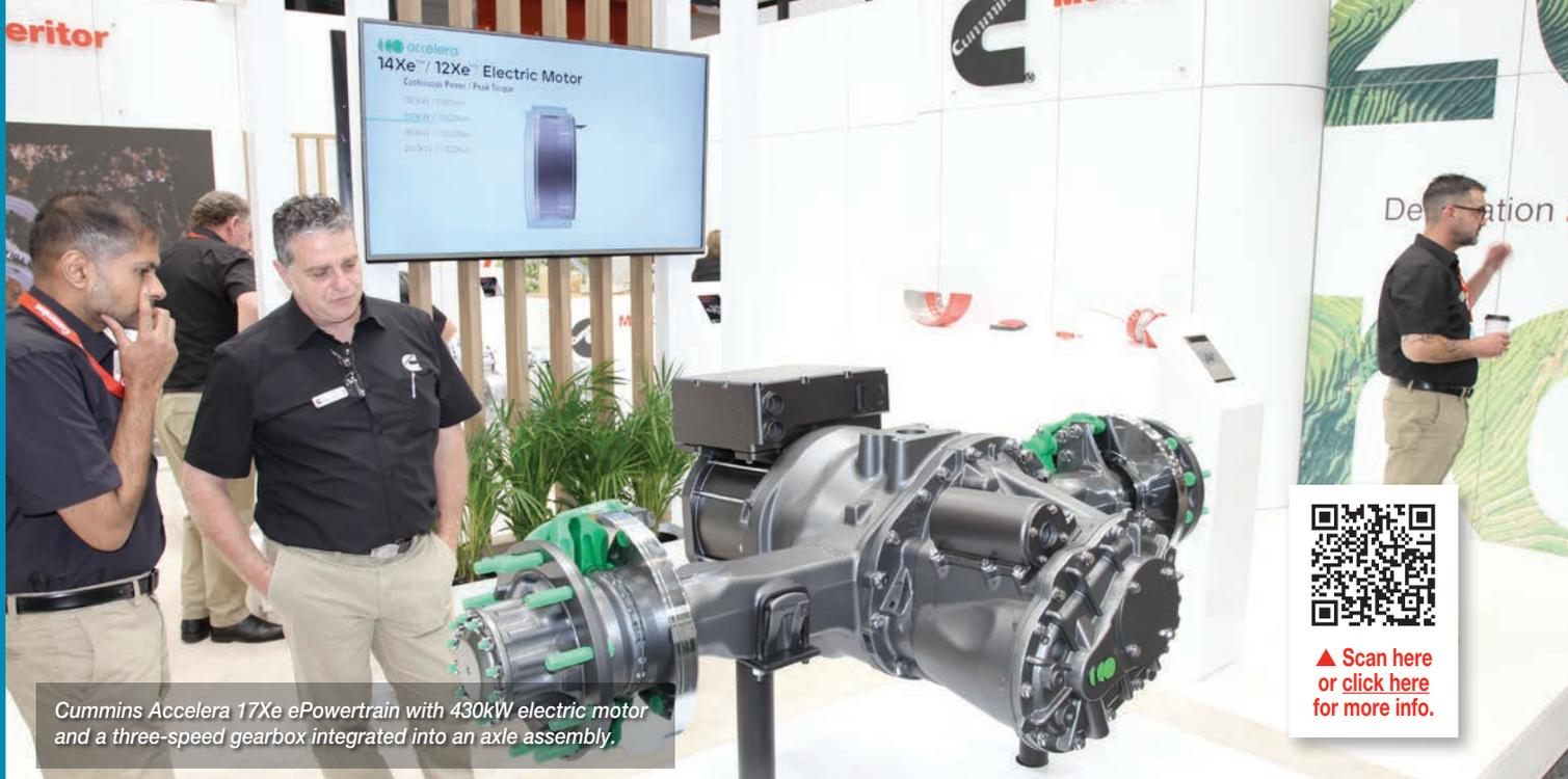
Cummins Accelerera 17Xe ePowertrain with 430kW electric motor and a three-speed gearbox integrated into an axle assembly.
