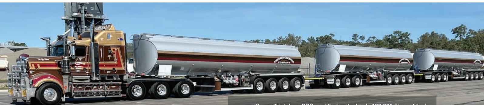
'Super Triple' – a PBS-certified unit – hauls 130,000 litres of fuel, a gain of up to 22,000 litres compared with a standard roadtrain triple.
