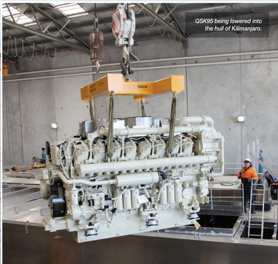
QSK95 being lowered into the hull of Kilimanjaro.
