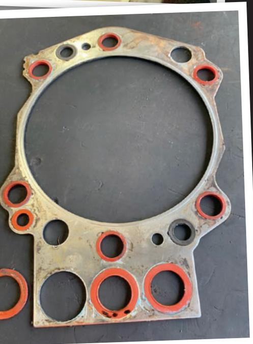
Some of the counterfeit parts that resulted in destruction of the 50-litre engine.
