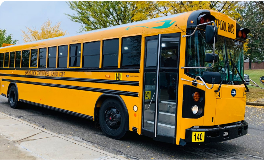
The next-generation electric school bus features the Accelera™ PowerDrive 7000 — the newest version of its electric powertrain system — with updated battery technology that has a capacity of 196kWh and can travel up to 130 miles on a single charge.
