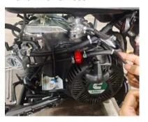
**10.** Remove the low pressure hose and the fuel hose by squeezing the clamp and pulling off.
