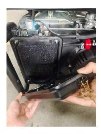
4. Remove the foam filter holder by removing the bolts.
