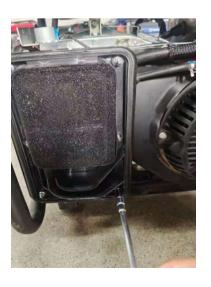
5. Remove bolt holding carbon canister rack and pull out.
