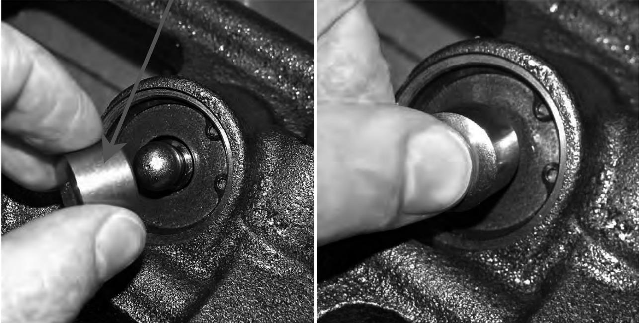
10. Place Item No. 6 E-Foot (Swivel Foot Assembly) over the ball of the Item No. 1 (Piston, Slave - Inner).
