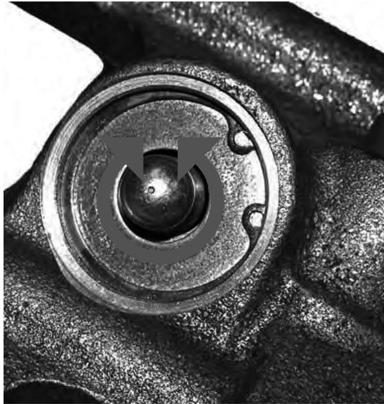
9. With the Tool Letter A (Slave Piston Clamping Tool) compressing the springs and washer, check that the Ring, Retainer 1.25 in. Dia. is in the groove by rotating the ring in the groove. See page 12 for the location of the groove.
