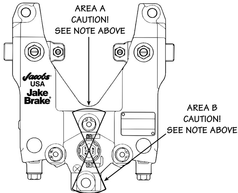
6. Torque the solenoid valve to 15 lb.-ft. (20 N•m) using a 3/4" socket.
