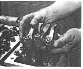
Remove rocker lever shaft holddown bolts and remove rocker shaft assemblies from the engine.
