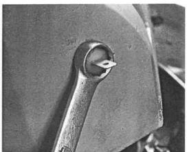
Connect the solenoid valve leadwire flag connector to the inside tab on the electrical terminal bushing.
