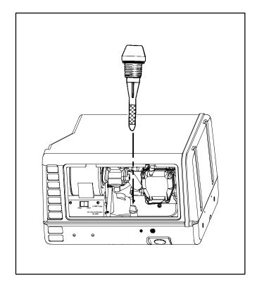
FIGURE 10. OIL LEVEL DIP STICK
