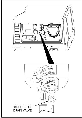
FIGURE 9. CARBURETOR DRAIN VALVE
