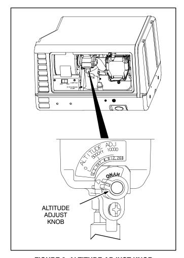
FIGURE 8. ALTITUDE ADJUST KNOB (GASOLINE MODELS ONLY)
