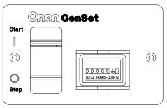
FIGURE 6. REMOTE SWITCH / HOUR METER
