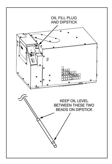
FIGURE 9. CHECKING ENGINE OIL LEVEL
