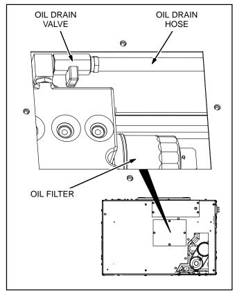
FIGURE 10. OIL DRAIN PLUG AND OIL FILTER
