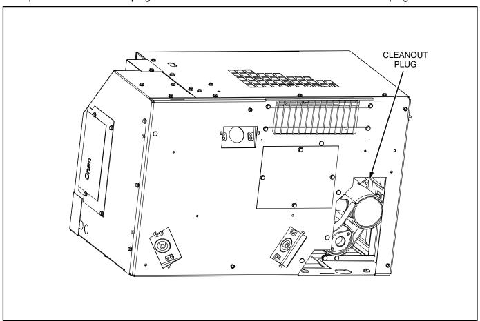
FIGURE 12. SPARK ARRESTOR CLEANOUT PLUG
