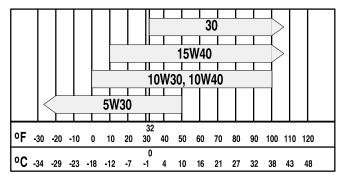
FIGURE 2. OIL VISCOSITY VS. TEMPERATURE
