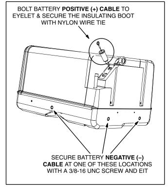
FIGURE 19. BATTERY CABLE CONNECTIONS
