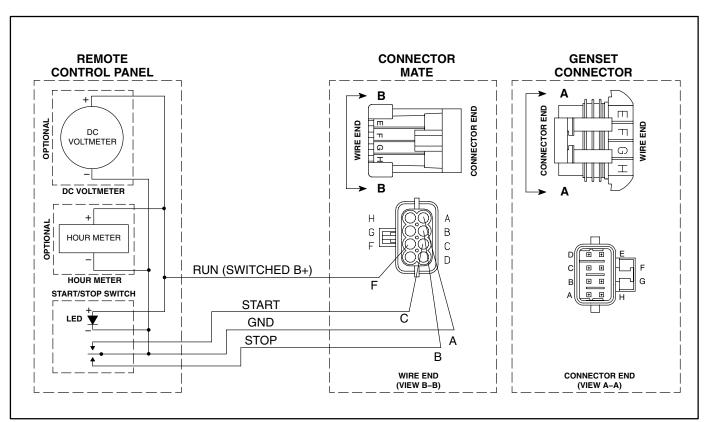
FIGURE 16. SCHEMATIC OF TYPICAL REMOTE CONTROL CONNECTIONS
