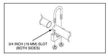
FIGURE 5. EXHAUST TAIL PIPE CONNECTIONS
