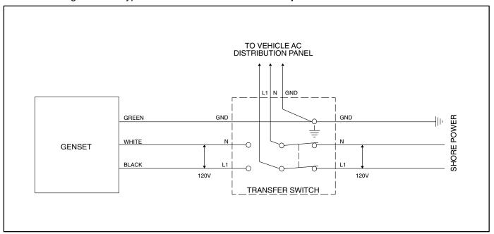
FIGURE 11. TYPICAL CONNECTIONS WITH TRANSFER SWITCH AND UTILITY
