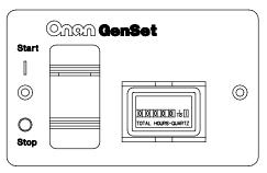
FIGURE 13. REMOTE SWITCH / HOUR METER
