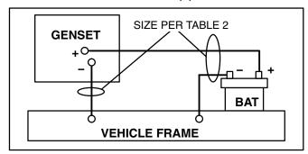
FIGURE 18. VEHICLE FRAME AS PATH FROM BATTERY NEGATIVE (-) TERMINAL
