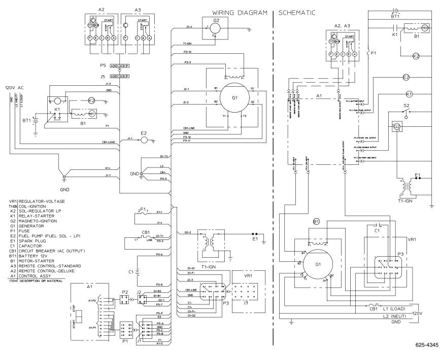
**60 HERTZ WIRING DIAGRAM AND SCHEMATIC**
