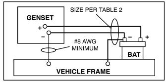
FIGURE 17. FULL-LENGTH CABLE FROM BATTERY NEGATIVE (-) TERMINAL
