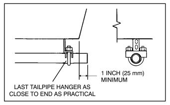
FIGURE 7. TERMINATING THE TAILPIPE
