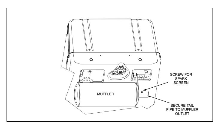
FIGURE 3. DIRECT-MOUNT MUFFLER FOR 60 HZ GENSETS ONLY
