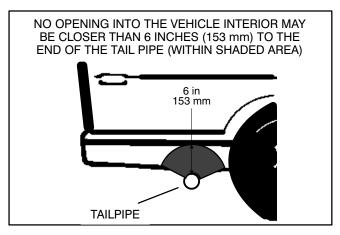
FIGURE 8. MINIMUM DISTANCES TO OPENINGS
