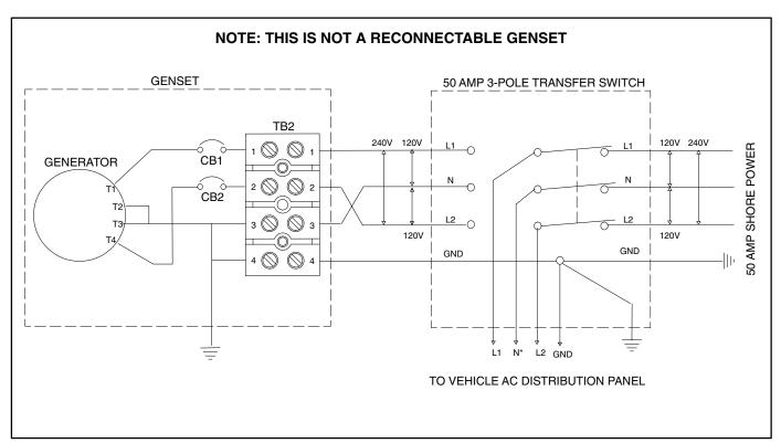
FIGURE 10. TYPICAL AC CONNECTIONS
