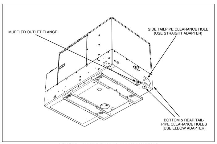
FIGURE 3. EXHAUST CONNECTIONS AT GENSET
