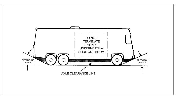
FIGURE 7. APPROACH AND DEPARTURE ANGLES AND AXLE CLEARANCE LINE
