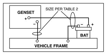
FIGURE 16. VEHICLE FRAME AS PATH FROM BATTERY NEGATIVE (-) TERMINAL
