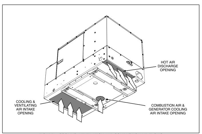
FIGURE 2. COOLING, VENTILATION AND COMBUSTION AIR FLOWS
