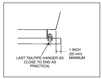
FIGURE 5. TERMINATING THE EXHAUST TAILPIPE
