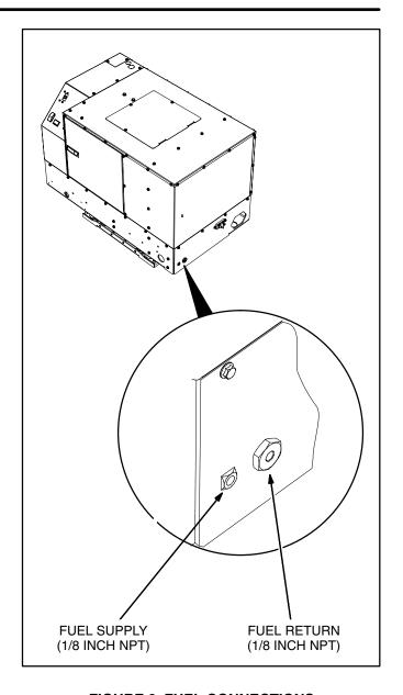
FIGURE 8. FUEL CONNECTIONS
