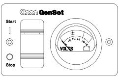
FIGURE 14. REMOTE SWITCH / DC VOLTMETER
