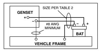
FIGURE 15. FULL-LENGTH CABLE FROM BATTERY NEGATIVE (-) TERMINAL
