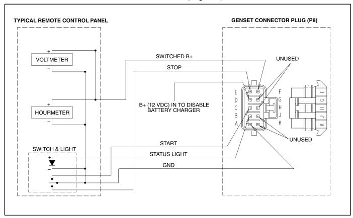
FIGURE 11. REMOTE CONTROL CONNECTOR PLUG AND TYPICAL CONNECTIONS
