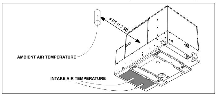
FIGURE 18. THERMOCOUPLE LOCATIONS FOR HOT AIR RECIRCULATION TEST
