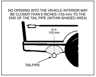
FIGURE 6. MINIMUM DISTANCES TO OPENINGS
