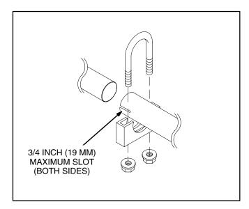
FIGURE 4. EXHAUST TAILPIPE CONNECTIONS
